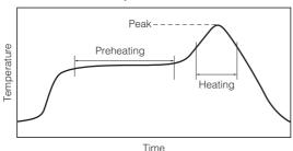
For soldering (Example: Sn/Pb)
